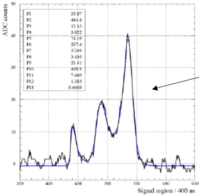
**Fitted signal shapes on single wire**
